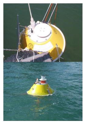
The buoy hull is manufactured from glass reinforced plastic (GRP) with stainless steel AISI316 inserts and internally filled with polyurethane foam. A rubber bumper is fitted around the buoy at water level. Eyebolts are provided for lifting, lowering into water and for mooring. The size and weight of the buoy Allow easy handling and transport. The hull holds up to 6 rechargeable sealed lead batteries (12V, 40 A/h each) giving 3.5 KW hours of reserve power.
