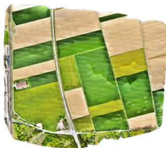
eBee X with Aeria / Delair UX11 Coverage 70 ha (173 ac) Altitude 57 m (187 ft)
