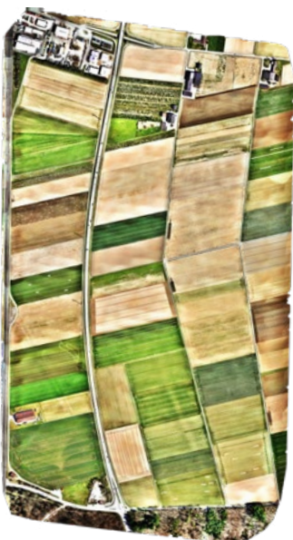
WingtraOne with RX1R II Coverage 110 ha (272 ac) Altitude 93 m (305 ft)
