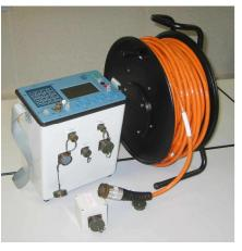
The SYSCAL Pro Switch units use segments (seg) of multi-core cable which are reversible and interchangeable.
