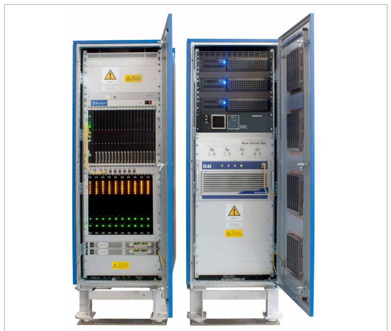
ELAC SeaBeam 3020 multibeam sonar electronics
