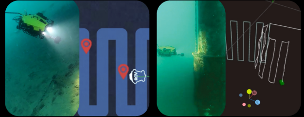
Mission Planning & Location-Tagged NDT Inspection
