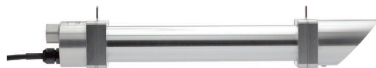
Figure 1 GEO-DR01 pyrheliometer: (1) humidity indicator, (2) sights, (3) aperture tube, (4) protection cap, (5) window with heater, (6) cable gland, (7) cable
