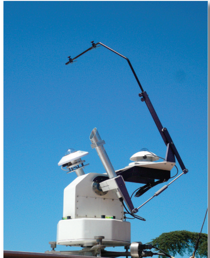
Meteorological Station with SunTracker-3000
